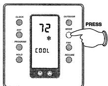
Step 2: Press and release the PROGRAM button – "Mo Tu We Th Fr"; Morning "\_\_\_\_" event symbol; and flashing starting time you programmed will appear on the display.
